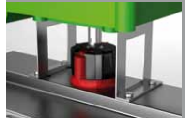
Namur connection for direct mounting switch box
