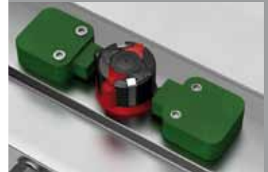
Mechanical switches indicating open and close
