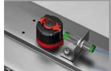
Inductive switch indicating open or closed position
