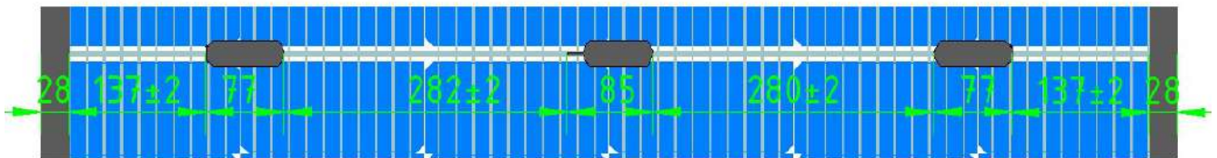
Figure 16. Position of the junction box in Blackstar B.108 Series module
