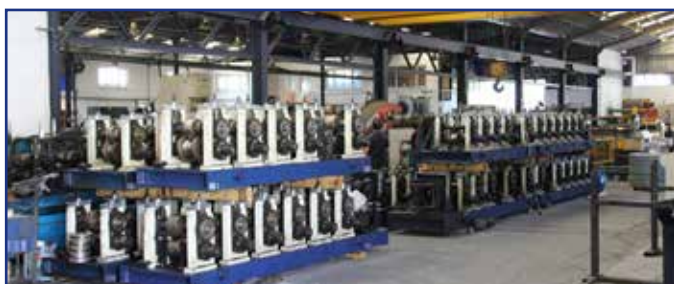
Profiling machines for production of anchor channels
